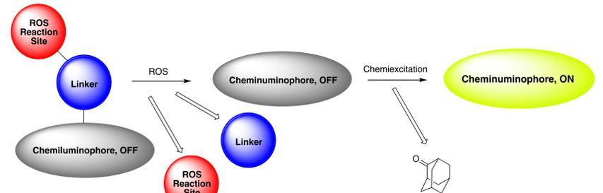
Scheme 3: General working principle of HOCl-DF-510 and HOCl-DF-540
